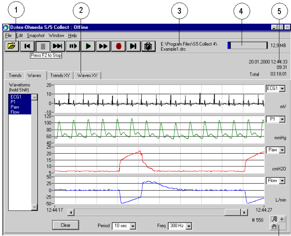
Figure 5-2 Example of the main window in offline mode
